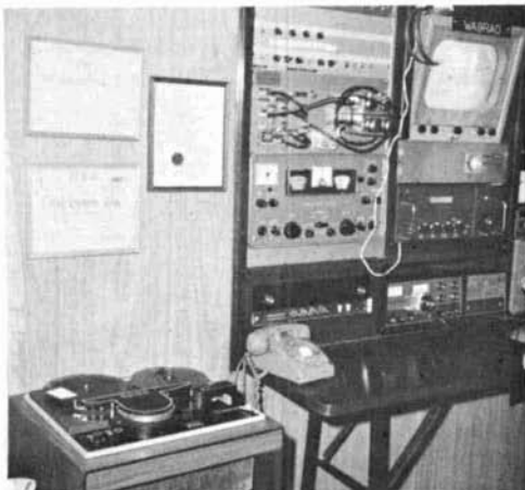
Author's home station is used for TV-DX as well as for amateur communications. Note CATV-type TV monitor in upper right.
